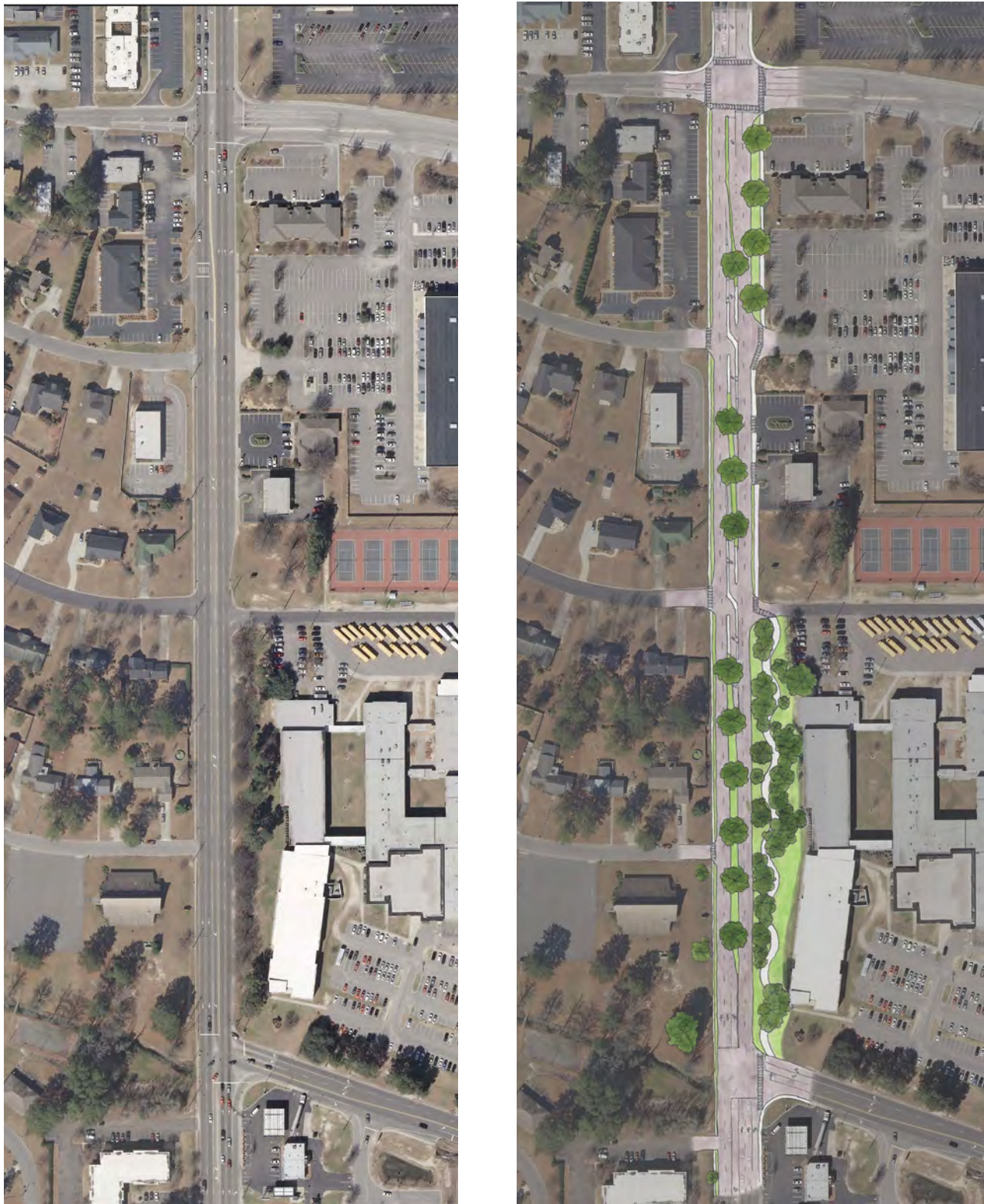
FIGURE 4.6 This section of Fayetteville Road is approximately 60' wide with 4 travel lanes and a center turn lane. The conceptual improvements maintain the four travel lanes, while providing turning lanes at key intersections to reduce the number of potential conflict points and frequency of vehicular crashes.
