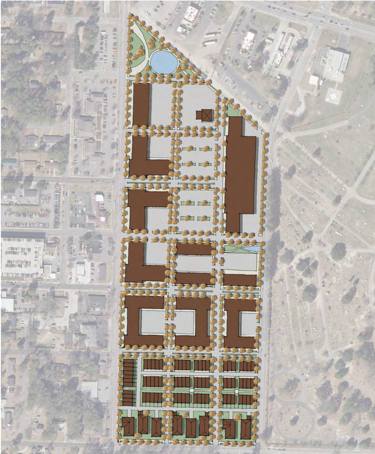
FIGURE 4.22 This concept drawing illustrates how the retail site could be redeveloped to include mixed commercial and residential uses utilizing a street grid that is consistent with existing, surrounding street patterns.
