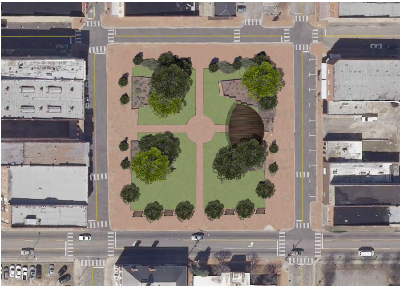
FIGURE 4.16 The above plan illustration of the plaza demonstrates the required changes that a two-way conversion would mean for this area. Signalized intersections would be required at North Elm and 2nd streets as well as North Chestnut and 2nd streets. Crosswalks at these intersections will unify the area around the plaza.
