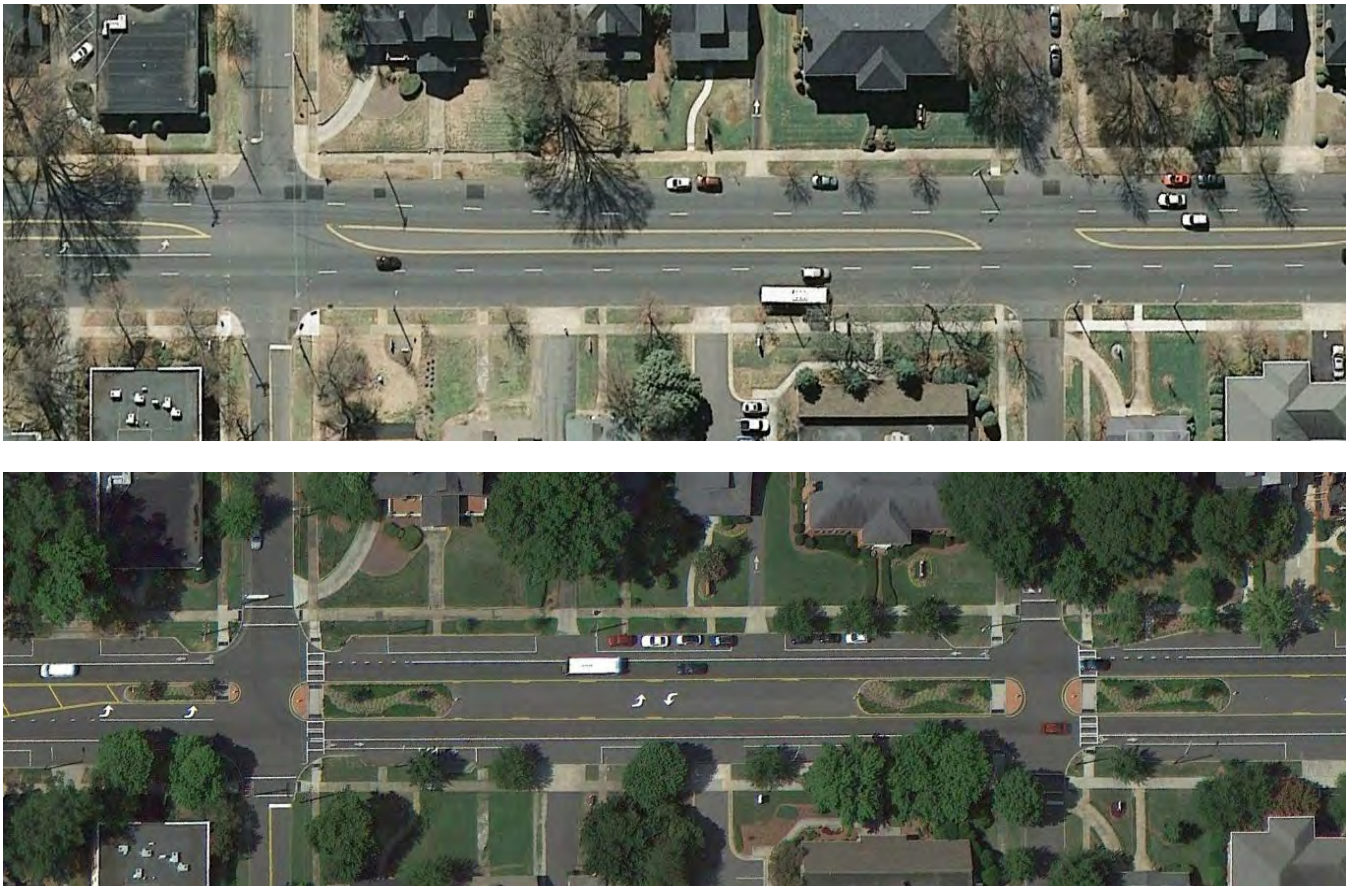
FIGURE 4.3 The above image shows the streetscape prior to complete street design improvements while the bottom image shows the streetscape with reduced travel lanes.
