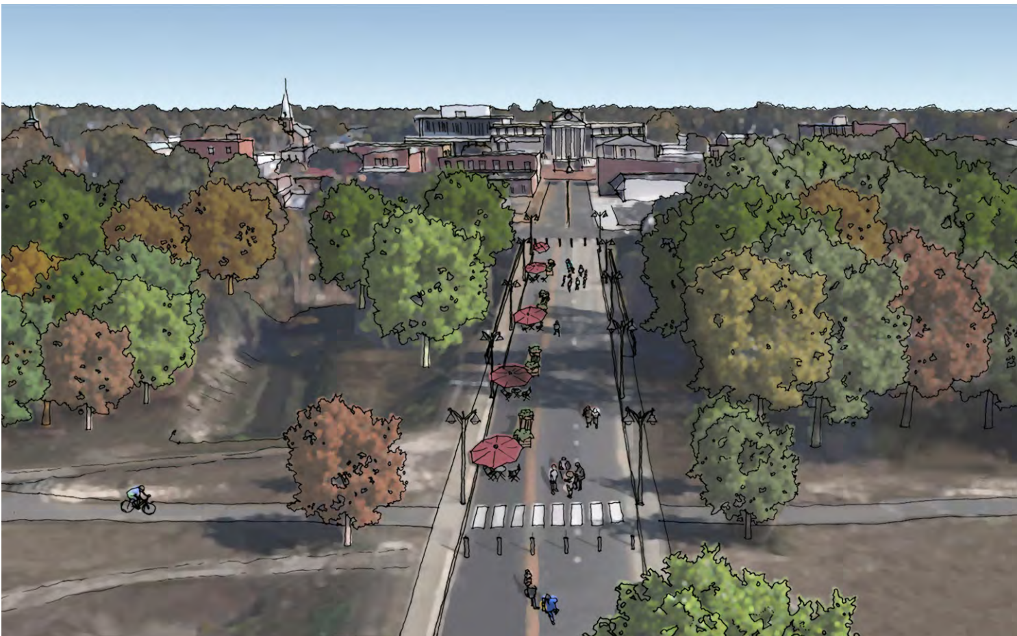
FIGURE 4.20 The image to the left is a bird's eye view of the 5th Street bridge into downtown. The below illustration demonstrates how the bridge park creates ease of access for pedestrians from the Riverwalk, across the Lumber River to downtown. Bollards can be removed during times of emergencies or infrastructure repairs.
